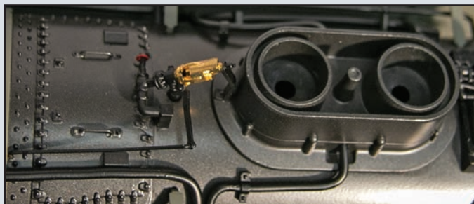
Operating smoke stack and whistle smoke - emits smoke when the whistle blows
