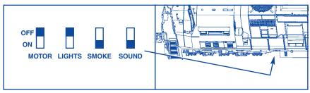
**CAUTION!** If the locomotive is going to be run for any period of time without smoke fluid, please position the smoke switch to the OFF position.
