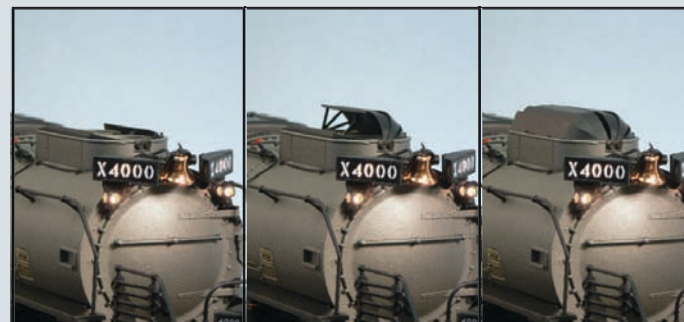
Detailed smoke deflector can be raised/lowered for prototypical operation
